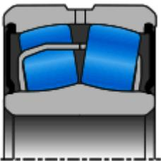
Do not use a product with a fibre glass reinforced polyamide cage over 150°C
