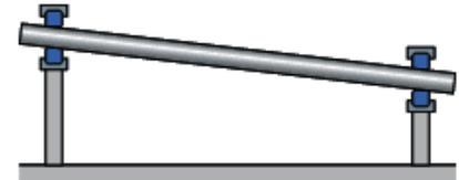
Shaft deflection creates misalignment between bearing inner and outer rings that is constant in magnitude and direction.
